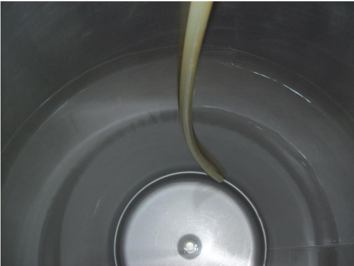
First installation step is to install the silicone tube onto the **out** port dip tube. Slide the tubing onto the dip tube at least 3/8". With a gentle tug, the tubing should stay put, if not, remove the tubing and dry the dip tube with a clean cloth. As you can see, the
