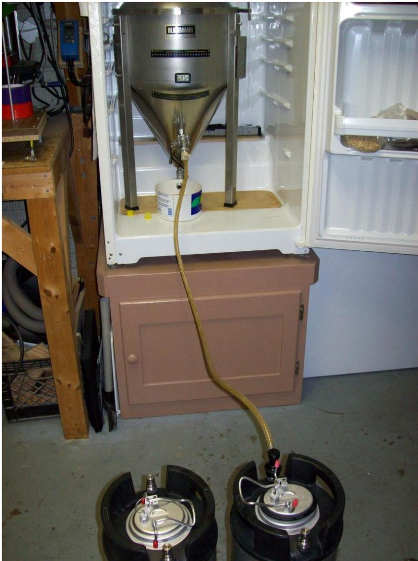
Gravity filling 2 kegs via the out port. This is the preferred method as it fills the keg from the bottom up, reduces the risk of oxidation, and keeps the silicone tubing full of the current beer during the carbonation process. But, whichever fermentation system you use, and however you chose to fill the keg, the Clear Beer Draught System will still do its thing and improve your enjoyment of the draught beer you created.
