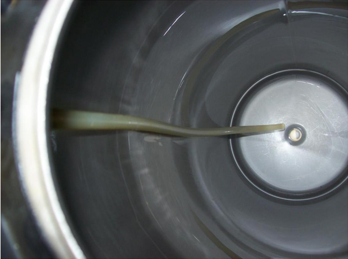
This is the correct positioning of the tubing. When hanging freely, the natural curvature points towards the center of the keg.
